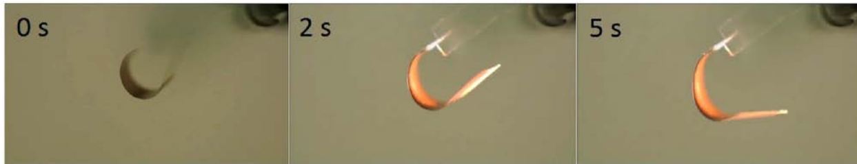
Figure 1. Typical photomechanical response of a-CN x film. The substrate is a 12- \mu m thick poly(ethylenenaphthalate) film.
