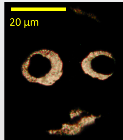
Transmitted light: Metal foil with glass halos at heated spots
