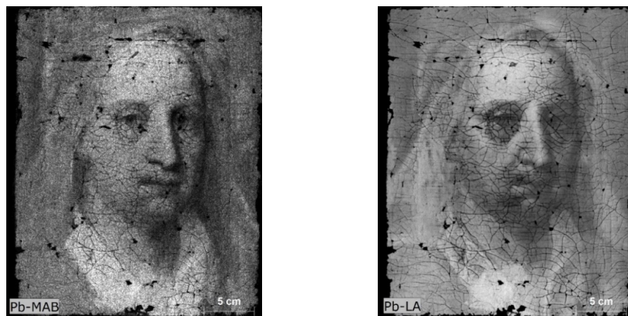
Figure 3. These element distribution images shown the distribution of lead in a painting. The first image shows the Pb-M lines at 2.4 keV and the second the Pb-L \alpha line at 10.54 keV. The difference in energies allows “display” of the element distribution at different depths. The L-lines show the painting down to the grounding, including the damaged areas on the left side, and the M-lines show the topmost thin layers of Pb pigments present at the painting’s surface.
