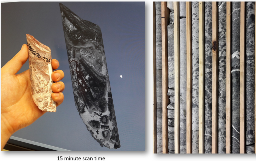
Figure 4. Example of a mineralised drill core taken from an exploration core tray and imaged rapidly using X-ray computed tomography technology (X-CT), to reveal 3D textural and mineralogical information without any damage to the sample.
