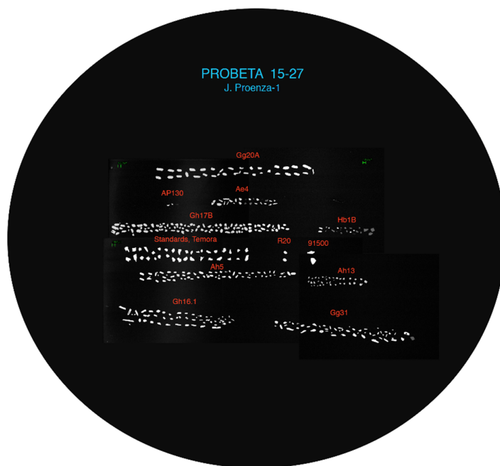
Figure 4. BSE image of a typical polished section ( d = 2.5 cm) as generally requested by dating laboratories with zircons from 9 different rock samples (and three standards) ready for geochronological measurements.
