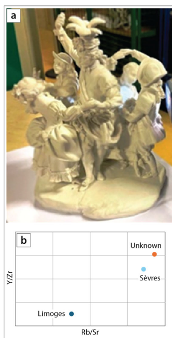
Figure 9. a) Sculpture produced using the biscuit technique, Sèvres Museum, Paris. b) Small-spot XRF point analysis of the ceramic sculpture compared to the composition of known manufacturing sources.
