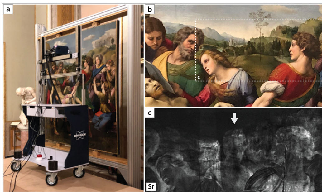
Figure 3. Illustration of the mobile capability of scanning \mu -XRF devices during a measurement campaign at the Villa Borghese, Rome. a) CRONO scanning XRF positioned for measurements in front of Raphael's "La Deposizione Baglioni". b) Visual image of a targeted area of the painting focusing on a region of landscape. (c) Elemental map (Sr) reveal the presence of a hidden figure (below arrow) now obscured by the landscape.
