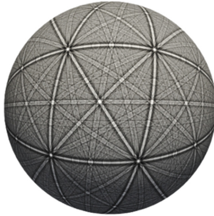
Figure 13. Simulated diffraction intensities on a spherical master pattern.
