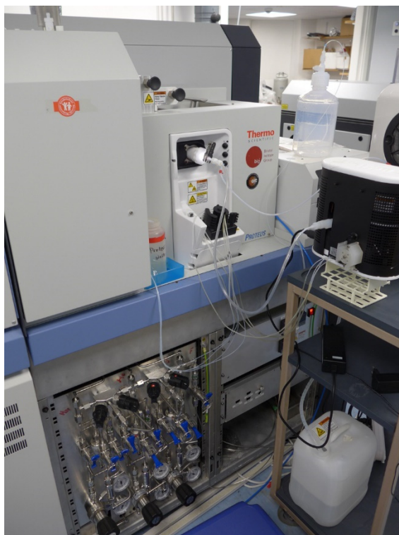
Figure 2. Photograph showing ‘front end’ of Proteus (top of screen), with sample line leading from Apex desolvator to torch, and gas delivery controls to collision cell (bottom of screen).
